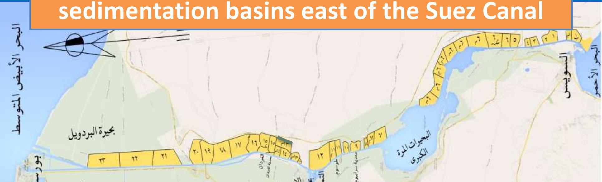
**23 Sedimentation Basins, totaling 120 km in length, and ranging from 3 to 5 km into the East bank of the Canal, extending from the bypass all the way down to the Gulf of Suez.**
